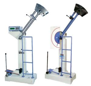
Accuracy conform to IS:3766-2003, IS:1598-1977, IS:1757-1999, IS:1499-2003, BS:131-Part- I, II, III, IV & BSEN-10045-1993 (for Charpy).
