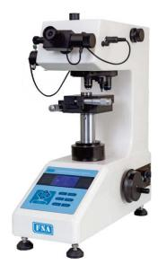
Extra (Optional) accessories like - Knoop Indentor, Knoop test block, Precision vice, Thin specimen holding device, V-shape anvil, Vertical & Horizontal fine specimen holding device, Rotary table, etc are available at an extra cost.
